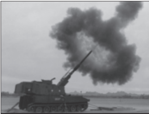
An M109A6 Paladin Self-Propelled Howitzer test fires an XM982 Excalibur 155mm projectile downrange at Yuma Proving Ground, AZ. The Excalibur's on-board guidance system will deliver the projectile within a 10-m CEP accuracy with a near-vertical, terminal angle, top-attack effects capability as demonstrated in this firing sequence. The Excalibur's increased accuracy also helps minimize potential collateral damage and civilian casualties when employed against point and high-payoff targets. (U.S. Army photo courtesy of PM CAS.)
