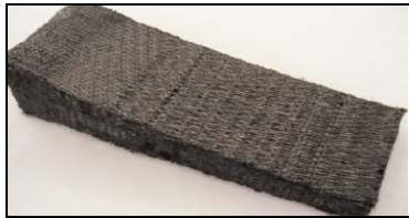
CF Woven Net Shape Preform (Techniweave)
