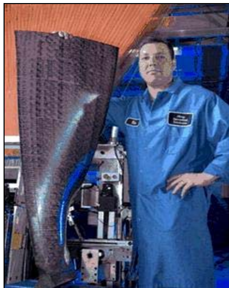
Densified CF Woven Preform (Techniweave)
