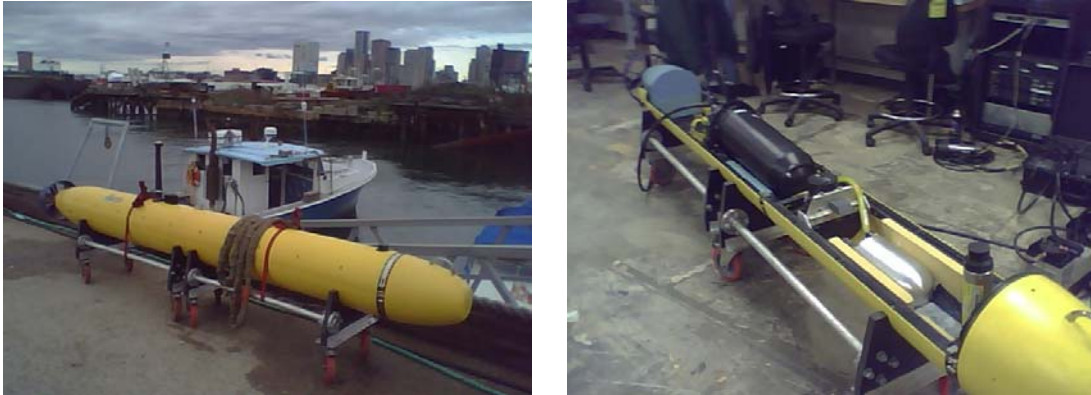
Figure 3. BF12 AUV photos taken during our November/December 2007 acceptance trials in Boston. The MIP payload consisted of the BlueView line sonar 3DLS (model MB1350), payload interface module (silver bullet), and ultra short baseline USBL tracking beacon.
