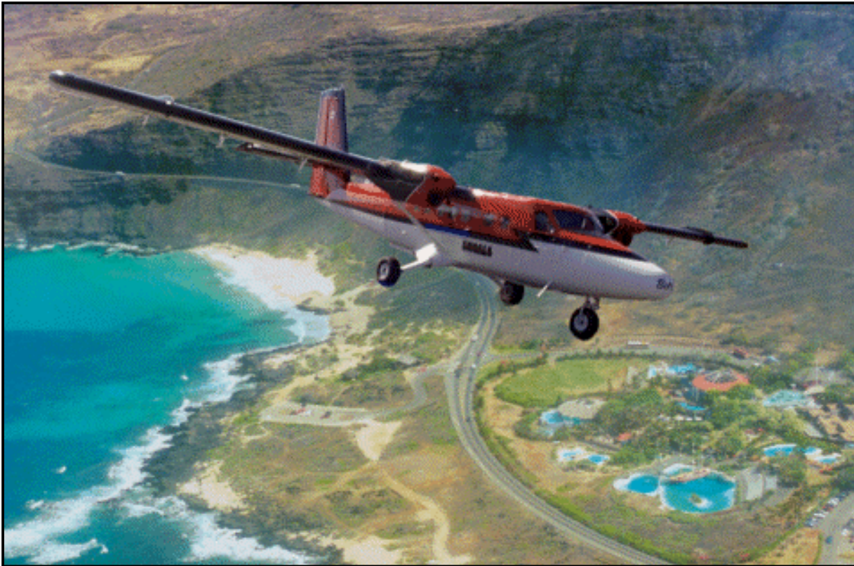
Figure 5 SHOALS lidar bathymeter in Kenn Borek Twin Otter over Hawaii.
