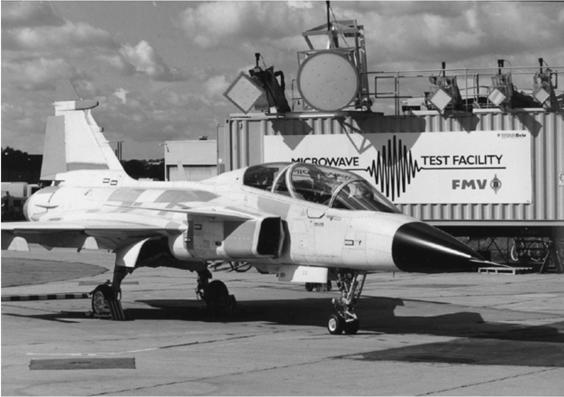
Figure 42. The Swedish MTF testing the HPM effects on Swedish Fighter Aircraft (Bäckström and Lövstrand, 2004)
