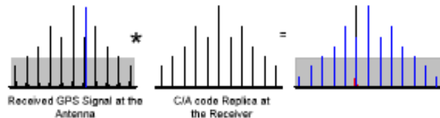
Figure 3 Code is despread by getting multiplied by the receiver code replica and interference is spread
