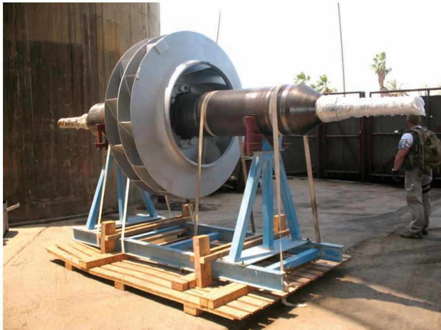
Rebuilt shaft for Unit 6 generator impeller.
