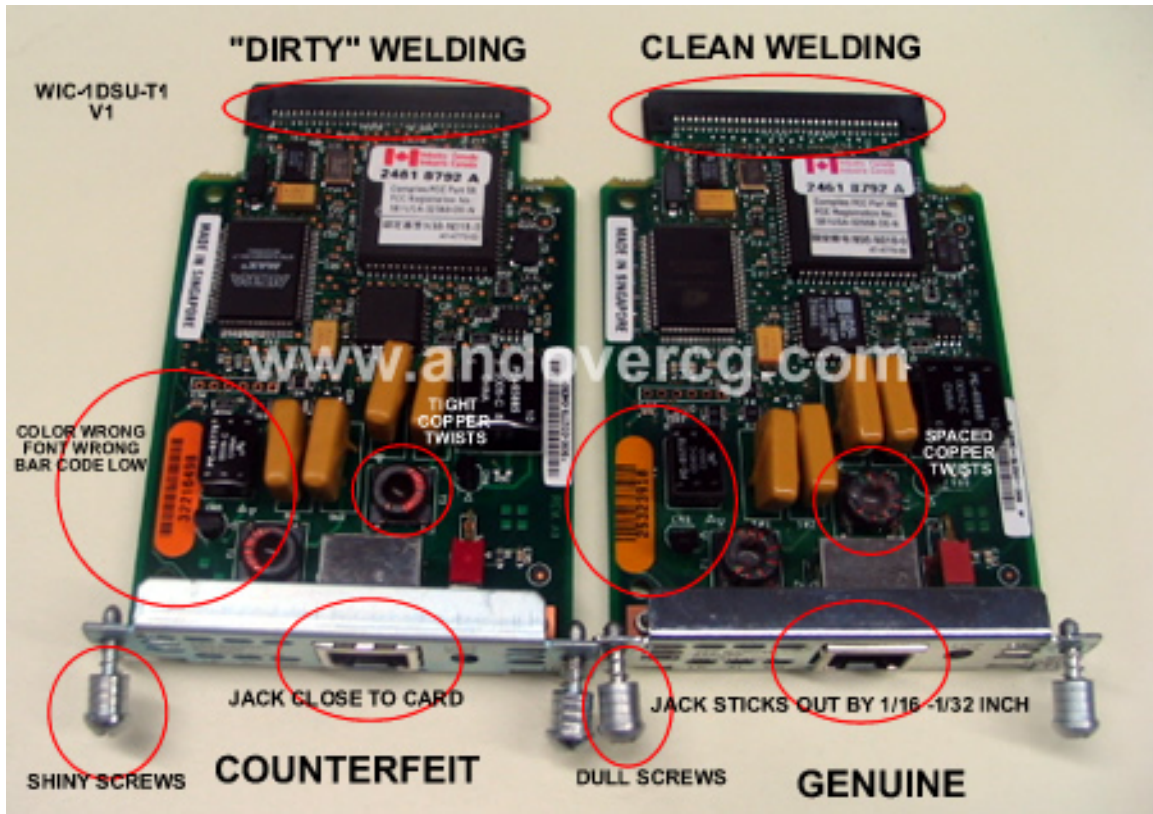
Figure 7. Counterfeit and genuine Cisco card (from: http://www.andovercg.com/services/cisco-counterfeit-wic-1dsu-t1.shtml ).
