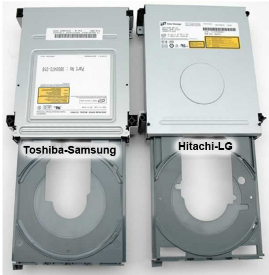
Figure 2. Photograph used to identify Xbox 360 DVD drives.
