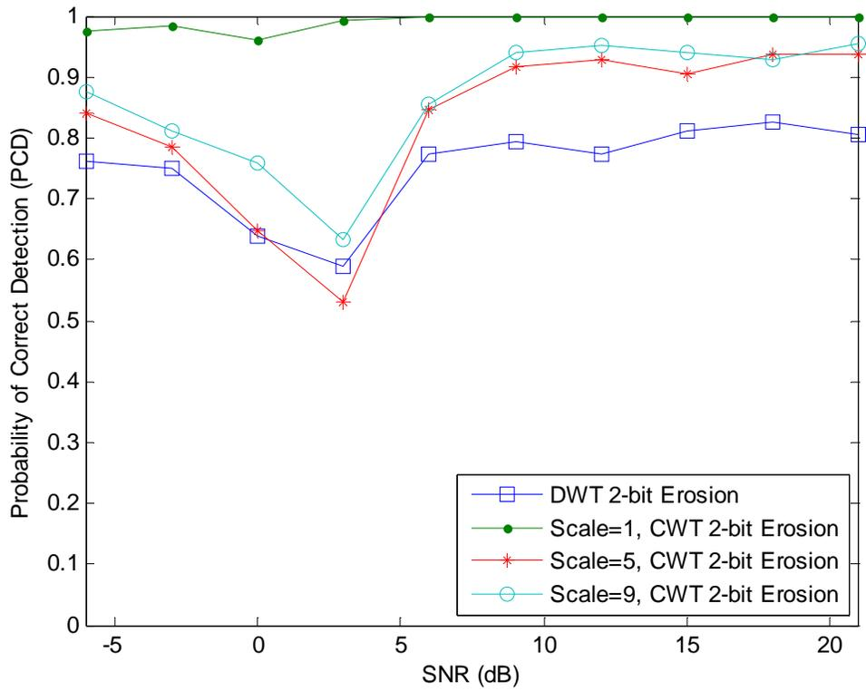
Figure 50. No-Hop Detection Performances for CWT at Different Scales and One-level DWT Transform, 2-bit Erosion Mask, 20% Detection Tolerance Level.
