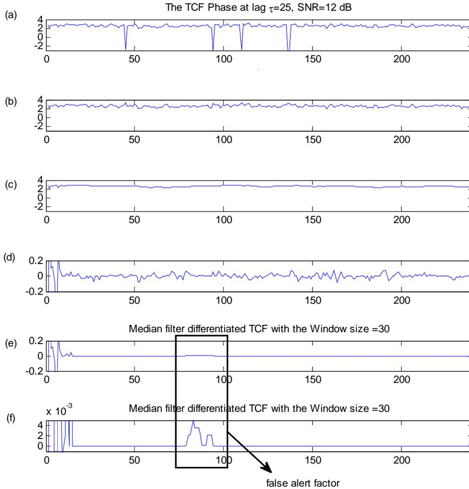
Figure 8. Impact Due to Successive Operations Applied to the TCF Phase for the No-hop Signal Case,  $TCF(t, \tau)$  for  $\tau = 25$  Fixed, SNR=12dB: First median Length=15, Second Median Length=30; (a) Original TCF Phase, (b) After Phase Unwrapping, (c) After Median Filtering, (d) After Differentiating, (e) & (f) After Second Median Filter.
