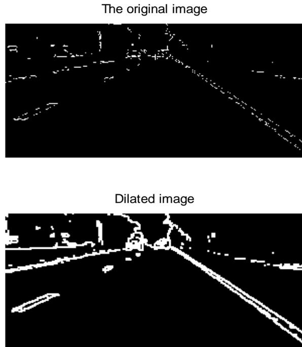
Figure 21. Dilation Operation Impact; 3-bit Radius Mask.
