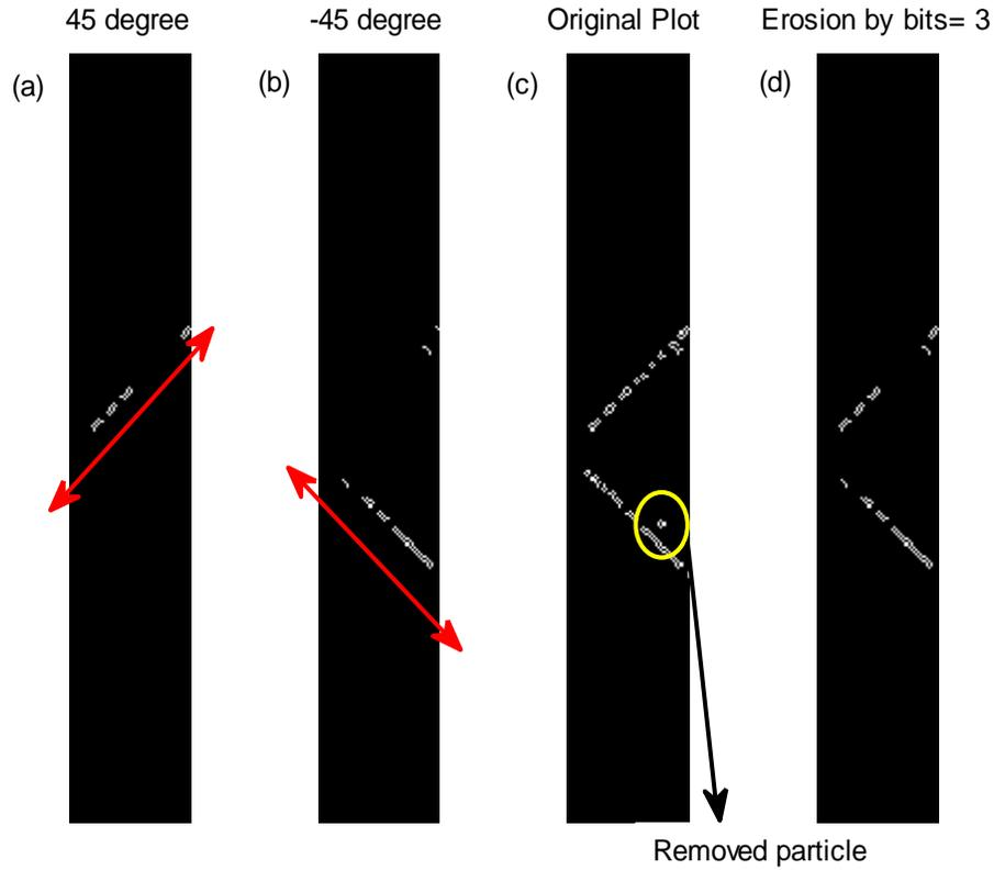
Figure 23. Erosion Operation of the Edge Detected TCF Phase Term with 3-bit Erosion Mask. (a) After 45° Mask Erosion; (b) After -45° Mask Erosion; (c) Original Plot; (d) Final Plot: Summation of (a) and (b).
