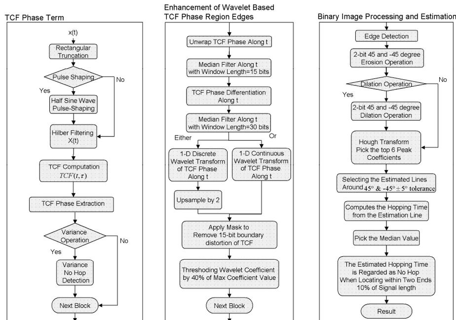
Figure 25. Overall FH Signal Timing Information Detection Algorithm Flow Chart.
