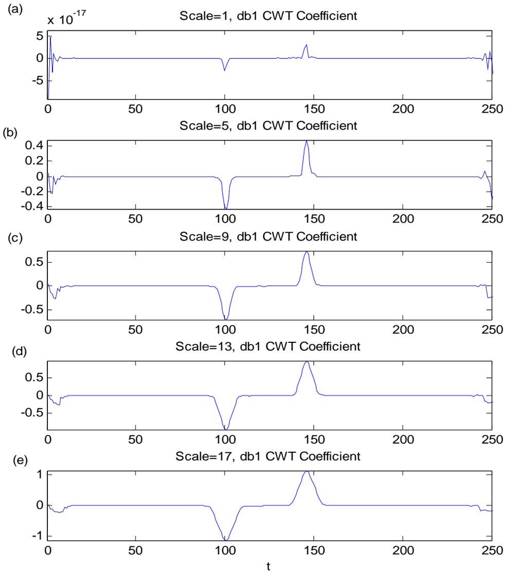
Figure 16. Application of the CWT to the Processed TCF Phase shown in Figure 15(a), (Haar Wavelet); (a) Coefficients for Scale=1, (b) Coefficients for Scale =5, (c) Coefficients for Scale =9, (d) Coefficients for Scale =13, (f) Coefficients for Scale =17.
