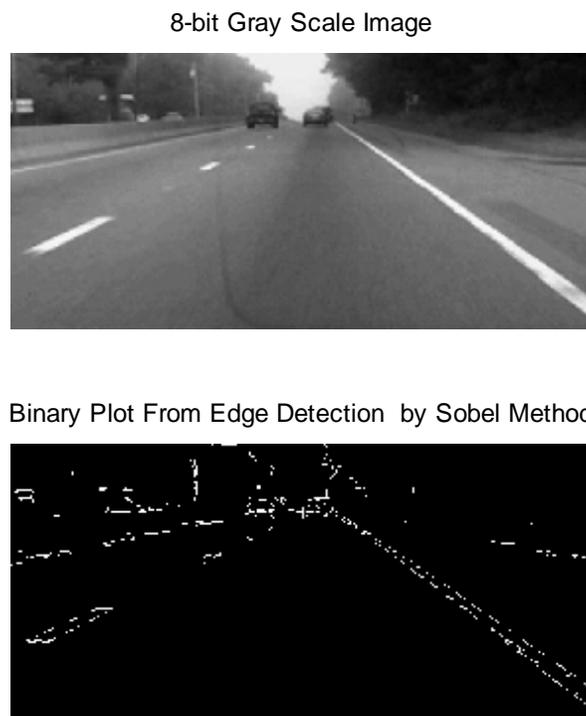
Figure 17. Edge Detection Using the Sobel Method, Operator Window Size Equal to 3.
