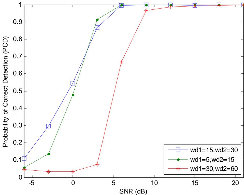
Figure 37. One-Hop Correct Detection Performance Results as a Function of the Median Filter Lengths; wd1: 1<sup>st</sup> Median Filter Length, wd2: 2<sup>nd</sup> Median Filter Length, 500 Trials per Simulation, SNR Levels Between -6dB to 21dB, 20% Tolerance Level.
