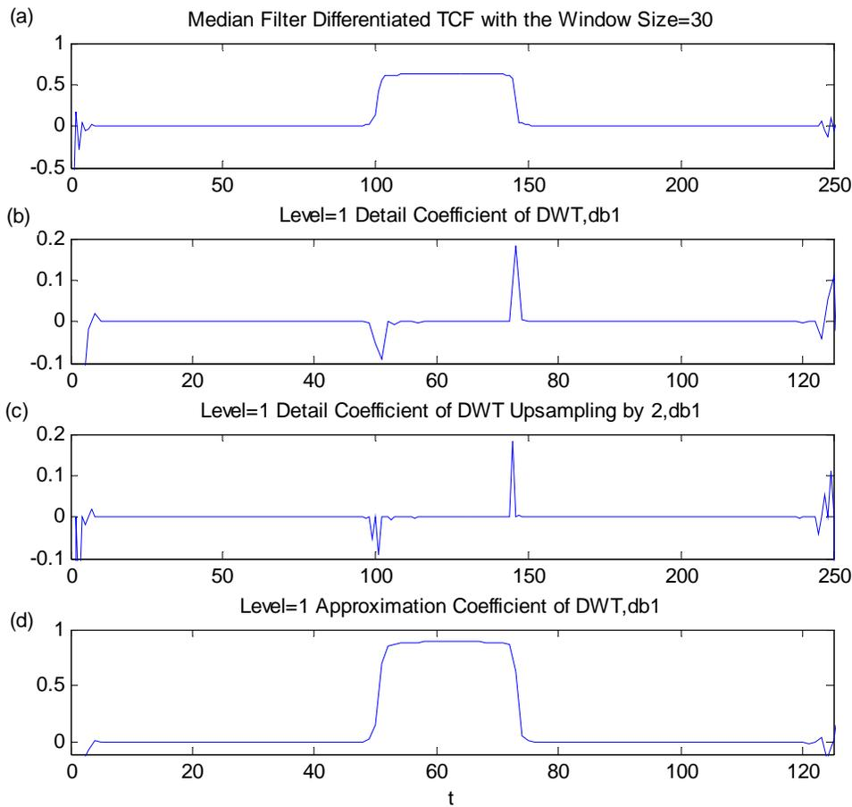
Figure 15. Application of the DWT to the Processed TCF Phase for a Fixed Lag Value  $\tau$ ; (a) TCF Function for a Fixed Lag Value (b) Detail Coefficients, One-Level DWT Transform of (a), Haar Wavelet, (c) Detail Coefficients after Up-sampling by 2, (d) Approximation Coefficients, One-Level DWT Transform of (a).
