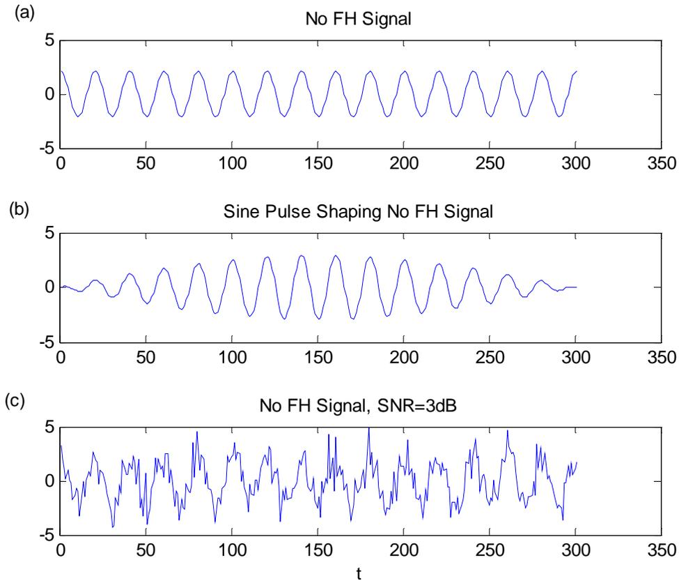
Figure 27. No-Hop FH signal. Basic FH Signal (no pulse shaping). (b) FH Signal with Sine Pulse Shaping. (c) Basic FH Signal, SNR=3dB.
