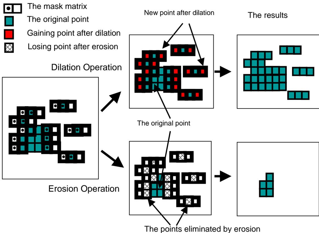
Figure 20. Morphological Operation; 2-bit Landscape Alignment Mask [After 10].
