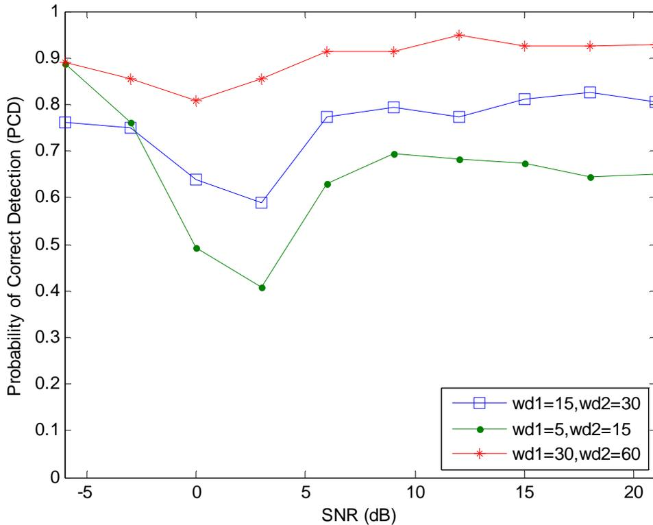
Figure 38. No-Hop Correct Detection Performance Results as a Function of the Median Filter Lengths; wd1: 1<sup>st</sup> Median Filter Length, wd2: 2<sup>nd</sup> Median Filter Length, 500 Trials per Simulation, SNR Levels Between -6dB to 21dB, 20% Tolerance Level.
