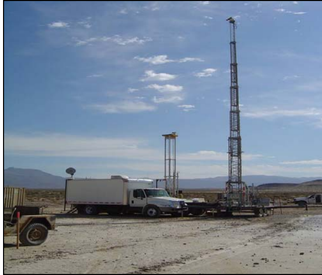
Figure 4. Laser support van and two towers used to support laser scoring instrumentation. Note the mobile tower and base.
