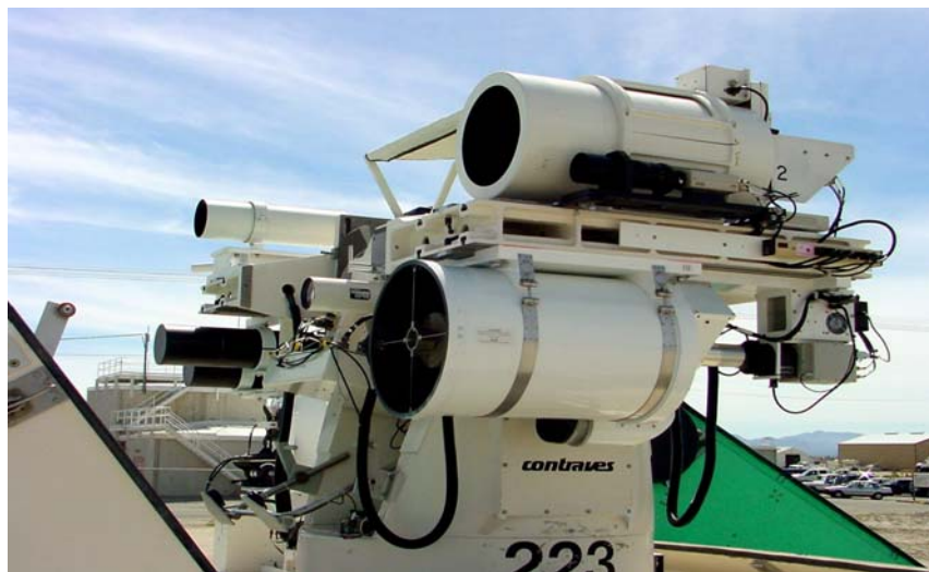
Figure 2. One of 15 Kineto Tracking Mounts (KTMs) with instrumentation cameras. KTM systems are mounted on trailers and towed from one location to another as needed.
