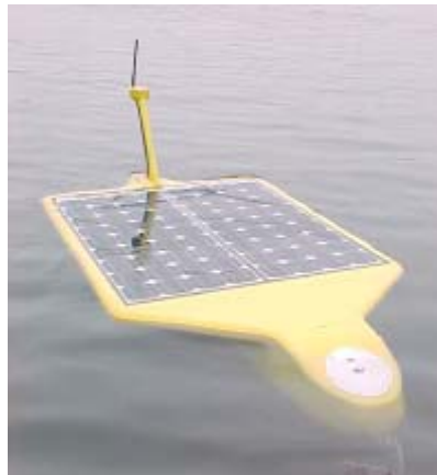
Figure 6. Solar-powered Autonomous Underwater Vehicle (SAUV). (from Jalbert, Baker, Duchesney, Pietryka, & Dalton, 2003)
