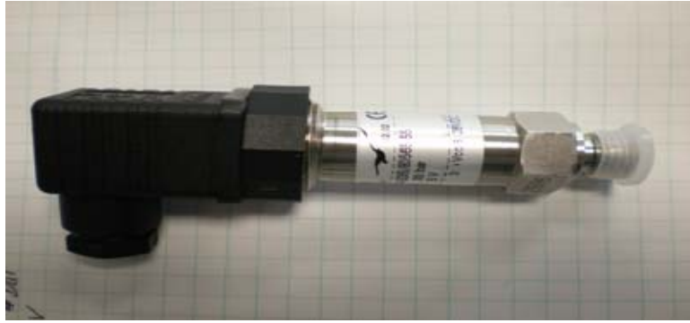
Figure 31. Keller-Druck Piezoresistive Depth Transmitter.
