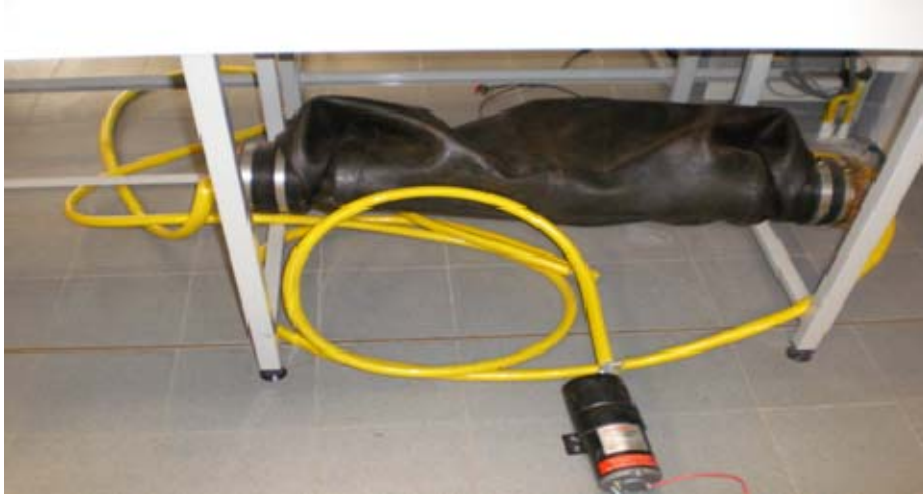
Figure 20. Expansion bladder for main ballast and associated tubing.
