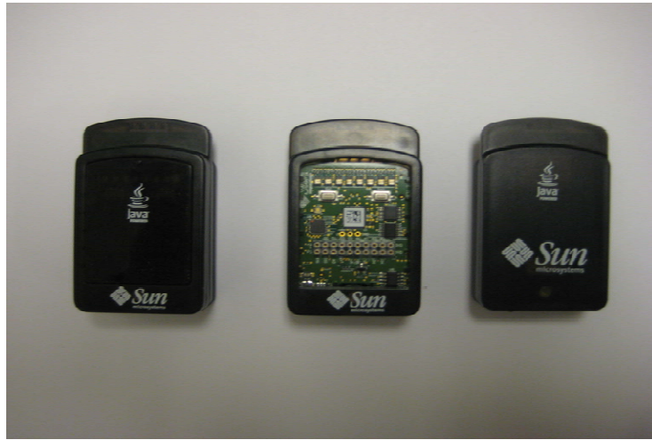
Figure 18. Free range Sun SPOT and base station.
