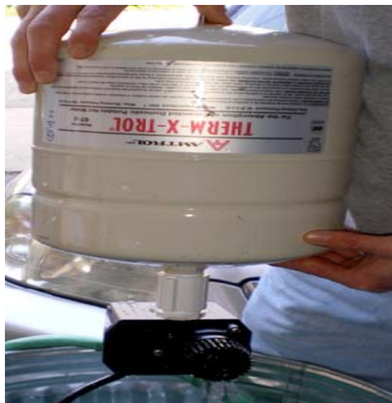
Figure 16. Submersible pump attached to expansion tank.
