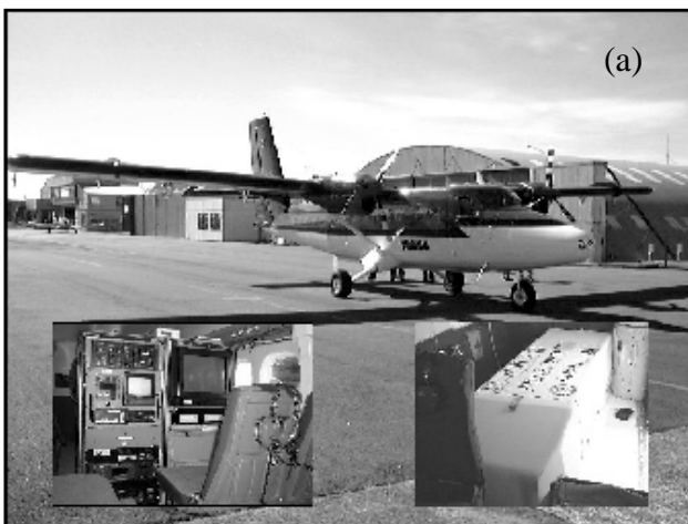
Figure 5. (a) SHOALS system mounted on a Twin Otter and (b) layout of SHOALS system inside Twin Otter.
