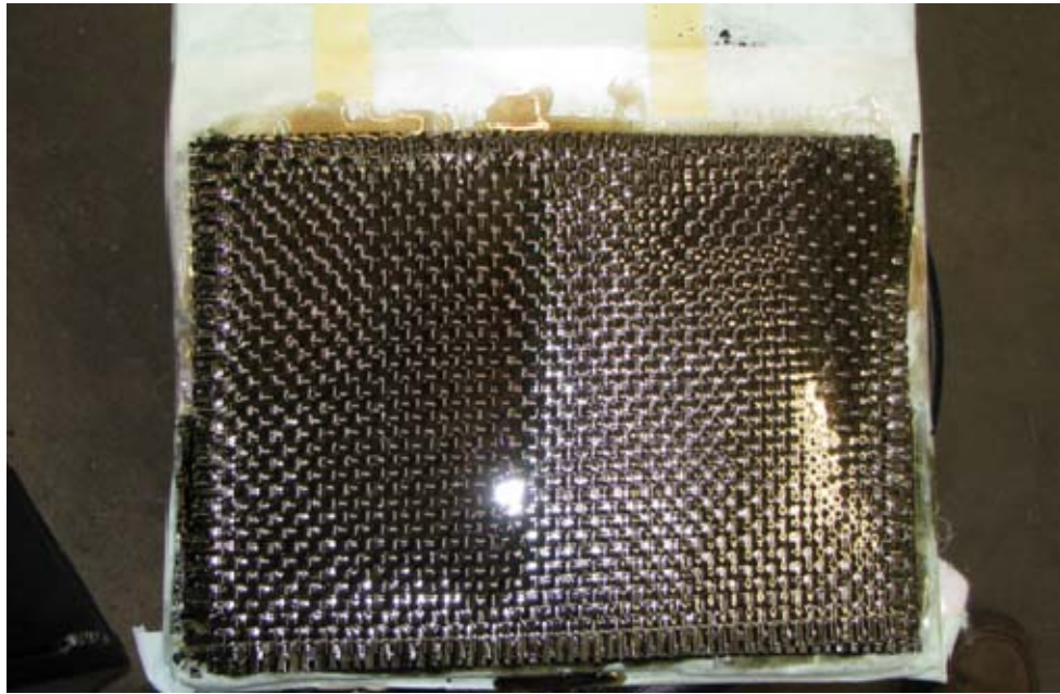
Figure 3. Image of composite sample prior to cure
