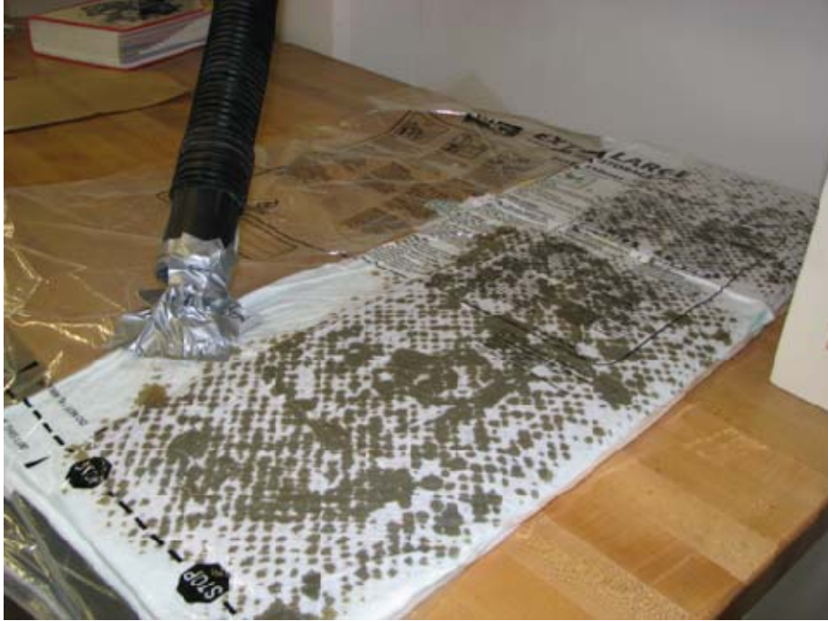
Figure 4. Image of composite sample curing under vacuum
