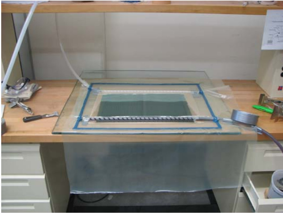
Figure 12. Resin flow through carbon fiber layers, showing inlet and outlet tubing
