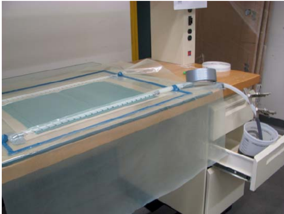
Figure 11. Vacuum applied during approximately 10- minute wait
