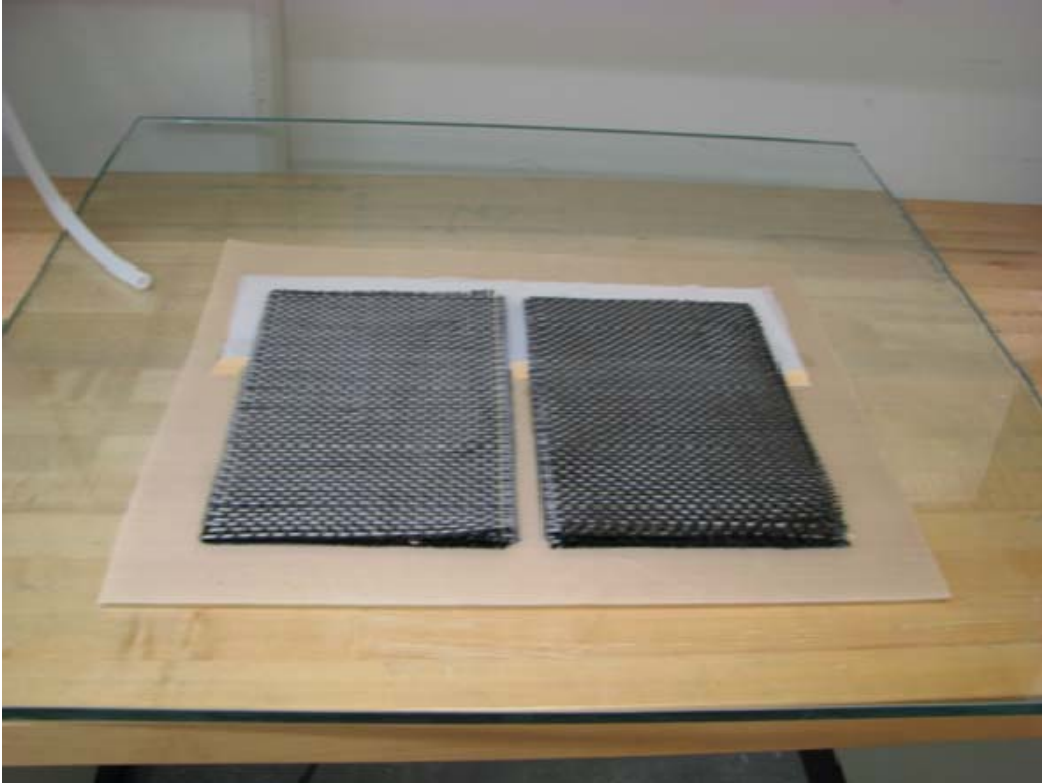
Figure 8. Layers of carbon fiber fabric stacked on peel ply
