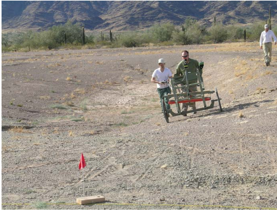
Figure 1. Demonstrator's system, EM61 MKII/pushcart.
