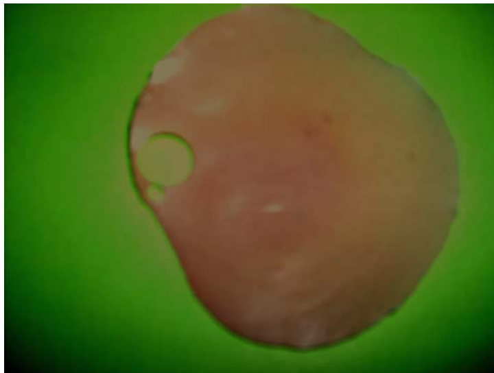
Figure 1. Typical appearance of a CP- and SZrO 2 -added PEO 20 LICF 3 SO 3 composite membrane.
