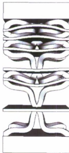
Fig. 4. The seven-layer truss panel after testing. (a) Experimental sample. (b) The numerical model with homogenized cores. (c) 3D unit cell model.
