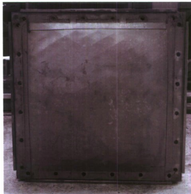
Fig. 5. Plan view of the back face after testing revealing minimal localized deformations around core members around the center.
