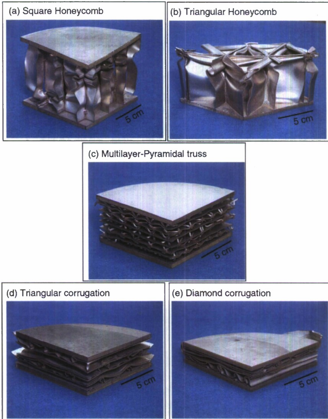
Figure 12: Photographs of the dynamically tested sandwich panels. The panels are sectioned along two orthogonal diametrical planes. (a) square-honeycomb, (b) triangular honeycomb, (c) multi-layer pyramidal truss, (d) triangular corrugation and (e) diamond corrugation.
