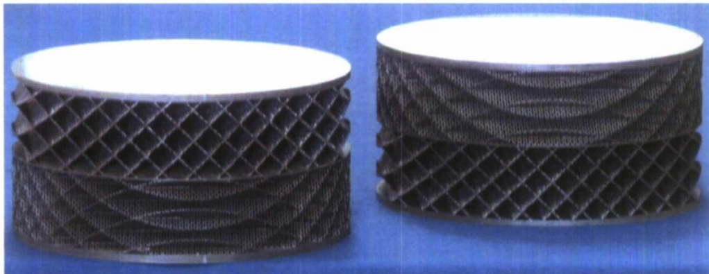
Figure 12 Woven wire mesh core, 8-inch diameter, “Dynocrusher” test samples. The wire diameter is 0.035”, and the wires are spaced 0.5” apart. The core relative density is 0.055
