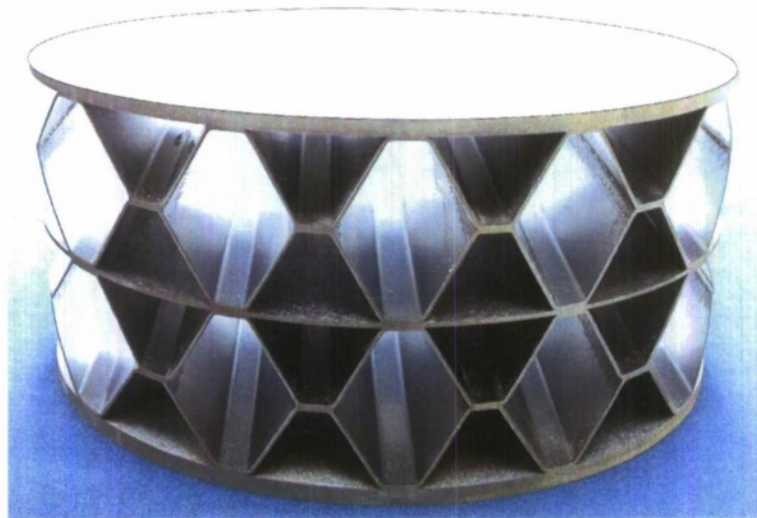
Figure 10. The double layer X-truss core dynocrusher sample with a core relative density of ~5.5%.
