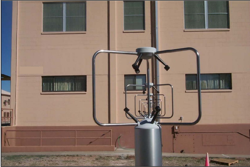
Figure 3. Photograph of the side-by-side sonic alignment during a relative calibration.
