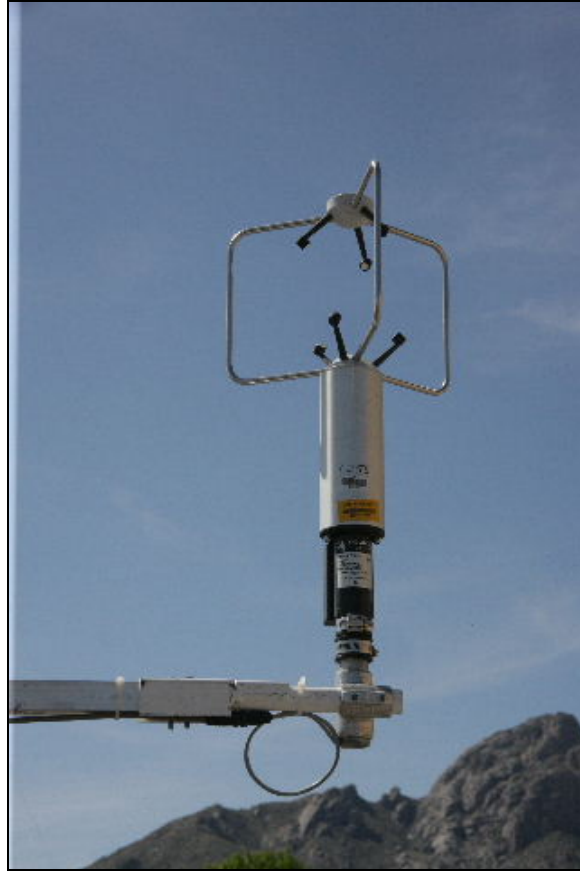
Figure 1. The RM Young 81000 Ultrasonic Anemometer was the primary sensor quantifying the dynamic character of the W07US urban site.
