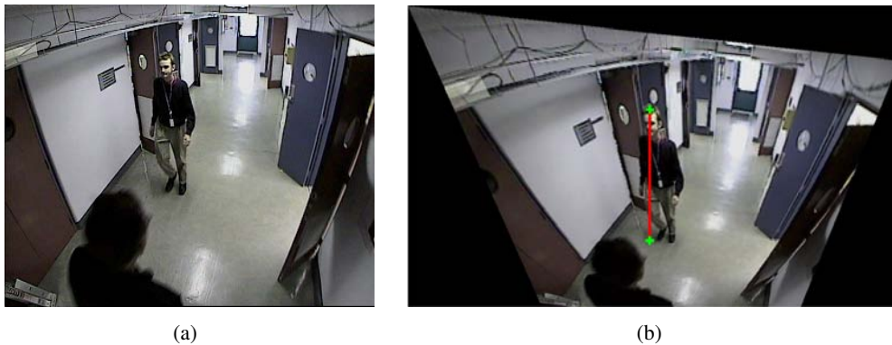
Figure 8: Image measurement from a surveillance camera. (a) Original image; (b) metrically rectified image with target segment.
