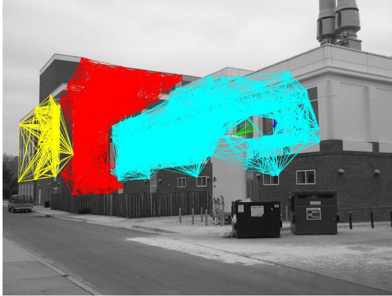
Figure 8. The final smoothed clusters of plane support points for the example image.
