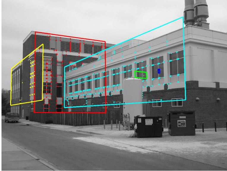
Figure 9. Building facades are determined by the vanishing point-aligned quadrilaterals that bound each smoothed cluster of support points.
