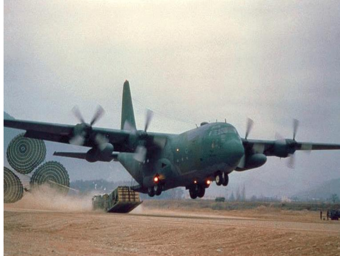
Figure 8: The C-130 performing a low altitude parachute drop
