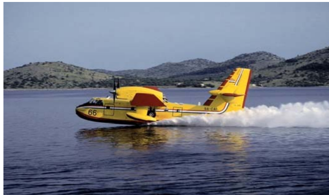
Figure 5: Canadair's amphibious CL-415 Bombardier with retractable landing gear
