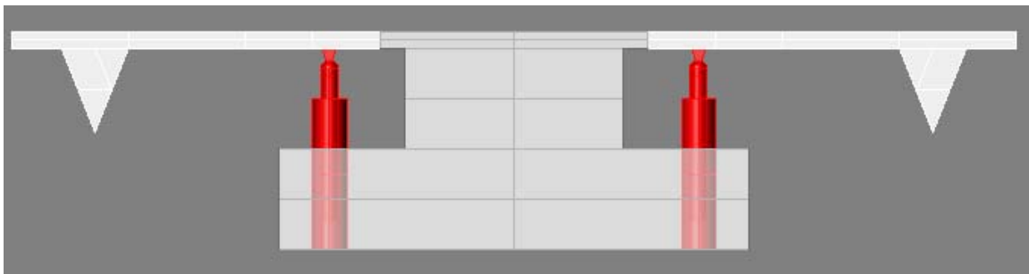
Figure 6. View of the extended transformable platform held in place by hydraulic actuators.
