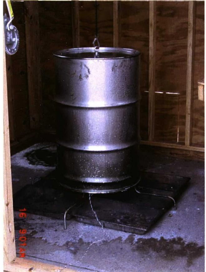
Figure 3. Grenade holding stand, drum, and sample pans used for smoke dissemination inside wooden shed. Left: four-legged stand with band-clamp and 55-gal placement and electric fuse wiring. Right: Placement of drum over the grenade for flare and pellet collection.
