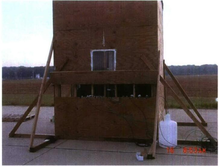
Figure 2. Wooden sheds used for smoke dissemination containment and sample collection (left), and with sample collection devices, jug, pumps, and tubing in place (right).
