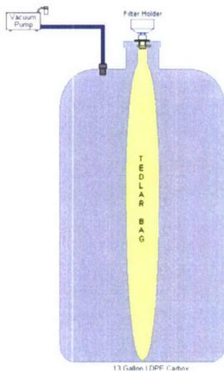
Figure 7. Experimental design for trapping inorganic gases.
