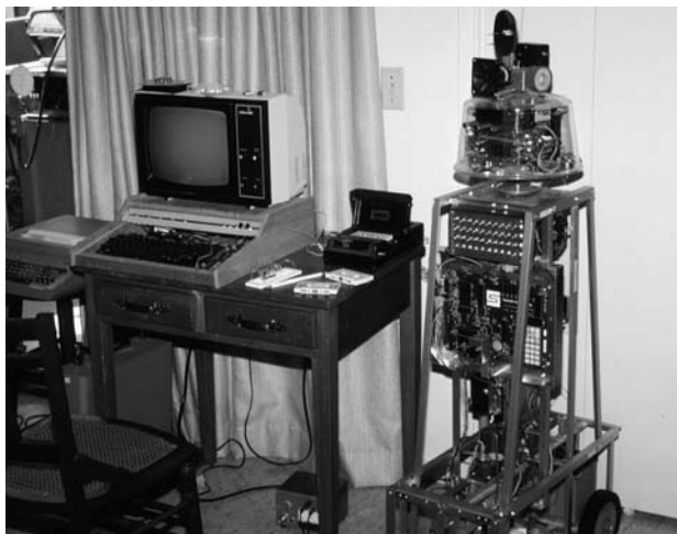
Figure 1-6. The Synertek KTM-2 terminal and a cassette tape storage system are shown beside ROBERT I , enabling the onboard SYM to be used for both software development and word processing (circa 1981).
