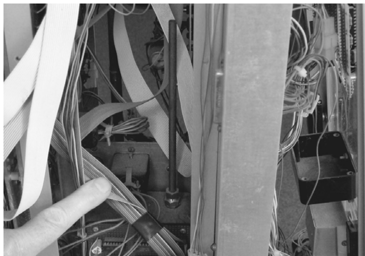
Figure 4-5. The earthquake detector (center) consisted of a free-floating rod inside a vertical brass tube, mechanically coupled at the base to a crystal microphone element.
