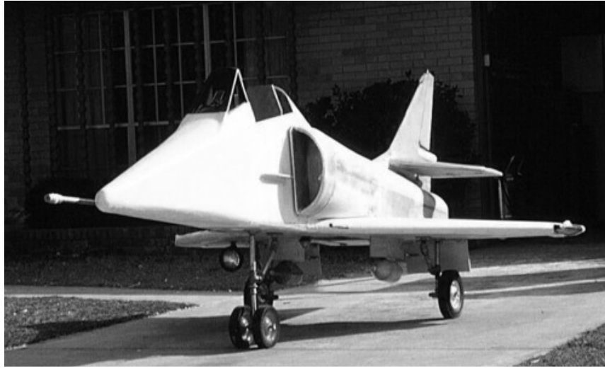
Figure 13. Front-quarter view during the early stages of fiberglassing. The landing light is visible under the starboard wing, and simulated bomb loads hang in the racks just inboard of the mainmounts, but the Sidewinder missiles have not yet been installed.
