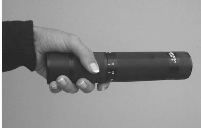
Figure 4-11. The Lifescan FLIR-6 , a handheld PIR human-presence sensor intended for law-enforcement use, was slowly scanned back and forth by hand to detect static targets.
