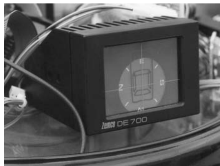
Figure 6-15. A Zemco DE 700 analog compass was used on ROBART II to determine the cardinal heading of a wall-following path segment.
