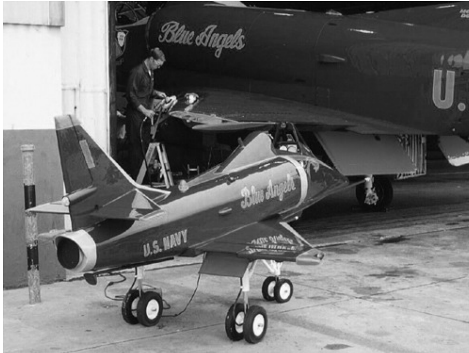
Figure 15. Once painted, the surface finish was smooth and shiny enough to where you could see your own reflection. Note the working tailhook below the rear fuselage, and the semi-functional instrument panel just visible in the cockpit.
