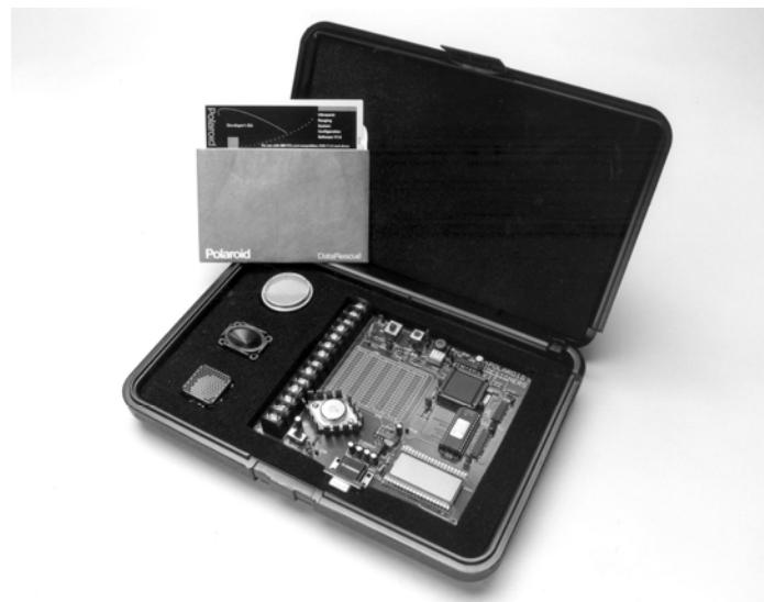
Figure 7-2. Introduced in 1982, Polaroid’s® ultrasonic ranging module would for the next decade become the sensor modality of choice for the mobile robotics research community. The more extensive evaluation kit shown above would later offer a range of transducers, but the original 1.5-inch sensor designed for camera autofocus remained the most popular (courtesy Polaroid Corporation®).
