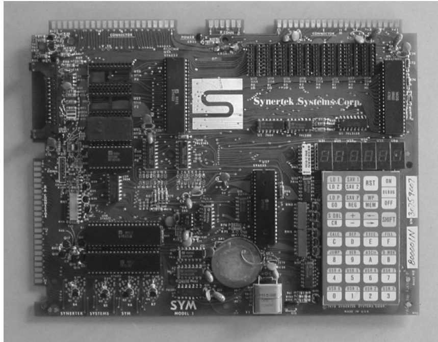
Figure 1-5. The Synertek SYM-1 single-board computer, introduced as a development kit for the 8-bit 6502 microprocessor, was rich in I/O capability and therefore ideal for robotic experimentation.
