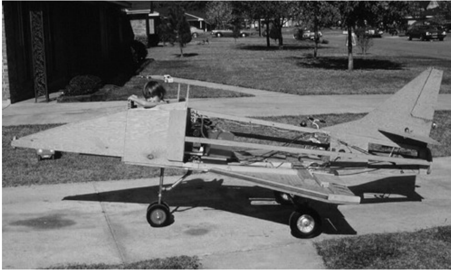
Figure 12. We first embellished by adding a three-dimensional fuselage structure atop the triangular wing, and closed in the cockpit and nose section as shown in 1/4-inch plywood.
