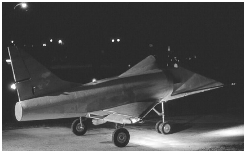
Figure 14. This hormone-inspired nighttime test of the cockpit, landing, navigation, and anti-collision lights was conducted with the simulated engine at full power, of course, just to convince the neighbors that we had really lost our minds.
