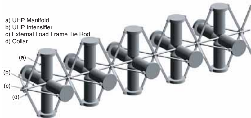
Figure 9. Illustration of Connection of Multiple Octahedral Modules to Make Up the Required UHP Gas Volume
