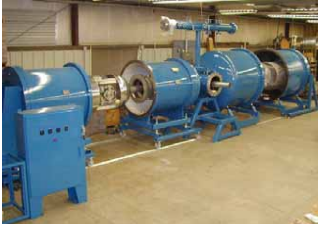
Figure 44. New 1-MeV Accelerator System for 5-ms, 1-s Blowdown Experiments at 1 MW, Shown Opened for Maintenance
