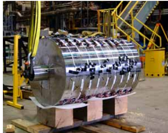
Figure 19. Completed A-2 Lite Pressure Vessel
