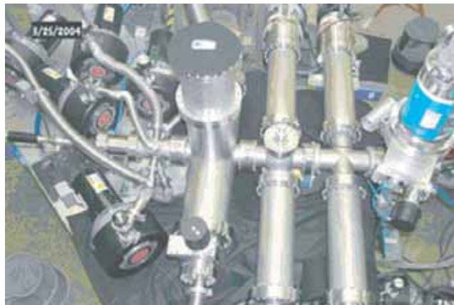
Figure 46. Differential Pumping Section that Forms the Vacuum Beam Window for Upcoming 1-MW, 1-s Blowdown Experiments
