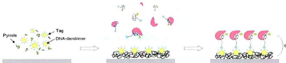
Fig 1: Illustration of aptamer based BoNT/A electrochemical detection
