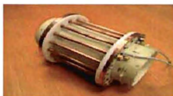
Fig.1 16-element double-tuned birdcage with Diameter=4" and Length=5"
