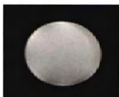
Fig.4 Proton image (a) and ^{13}\text{C} spectra (b) of a cylindrical corn oil phantom acquired using the double-tuned birdcage. Artifacts in (a) were caused by different chemical shift of protons in corn
