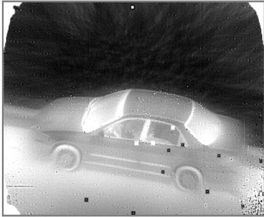
Figure 7a. MWIR data that has undergone spatial deconvolution. Frame 64.
