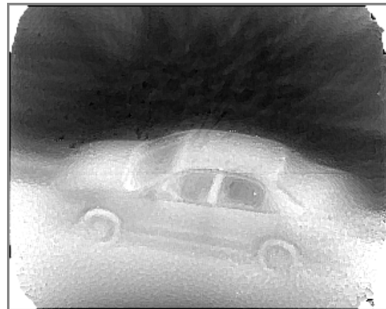
Figure 8b. LWIR data processed by a median filter and then spatial deconvolution. Frame 64.
