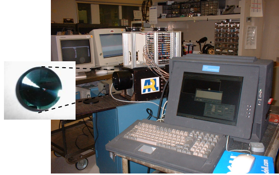
Figure 1. A photograph of DBHSI with expanded view of diffractive lens in the inset.
