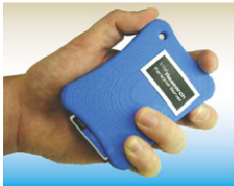
Figure 1. Prototype of an Intel XScale/Linux-based personal server (From: [2])
