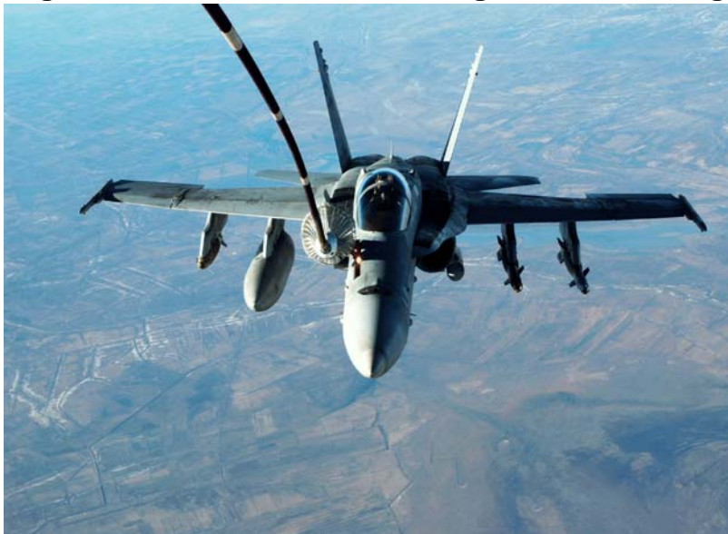
Figure 2. Photo of “Hose and Drogue” Air Refueling
