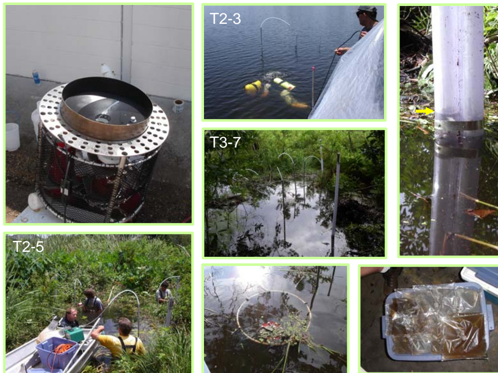
Figure 3-10. Field deployment and validation of the UltraSeep at three locations along Druid Lake.
