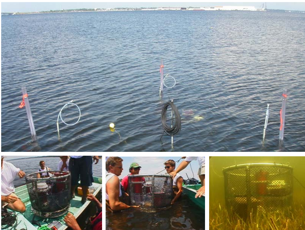
Figure 3-8. The UltraSeep being deployed in St. Andrews Bay (bottom left and center); installed on the bottom (bottom right); and viewed from above, including the array of VOC and level-logging piezometers at station T4-4 (top).
