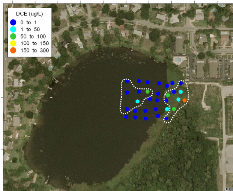
Figure 3-6. Trident probe sub-surface DCE map ( \mu\text{g/L} ) for the area offshore from OU 4. Dotted lines indicate groundwater discharge zones based on sub-surface temperature.
