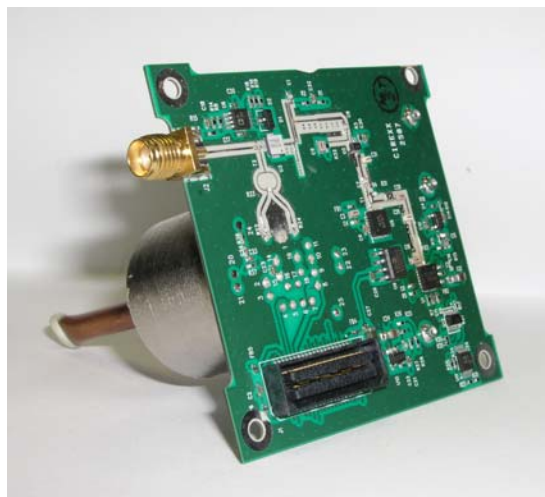
Figure 14. Initial integrated control electronics implemented with DSP servo control and an onboard RF diode-doubler/splitter.
