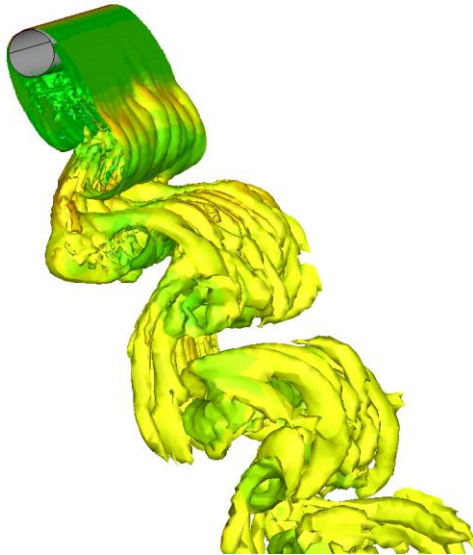
Figure 10. Instantaneous iso-surfaces of constant vorticity magnitude in the wake of the circular cylinder. Surfaces are colored by pressure.
