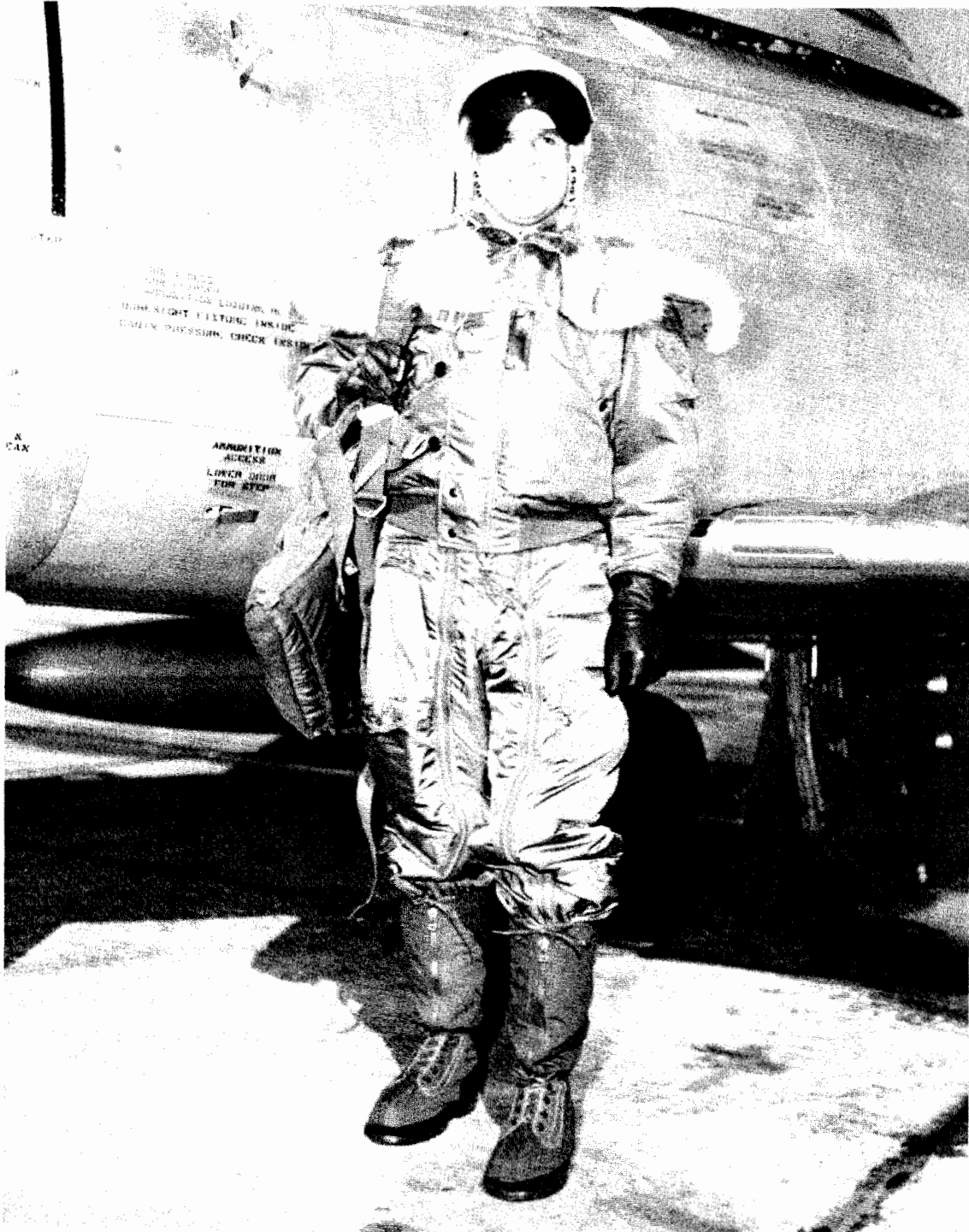
Fig III-38 High altitude flight clothing for jet aircraft, developed and tested by the Clothing Branch.
