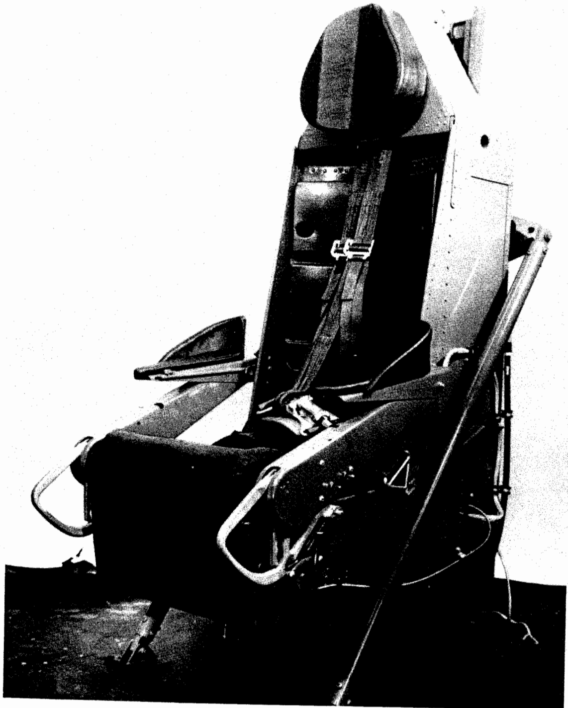
Fig III-39 The first tiltable ejection seat for long range jet flight missions.
