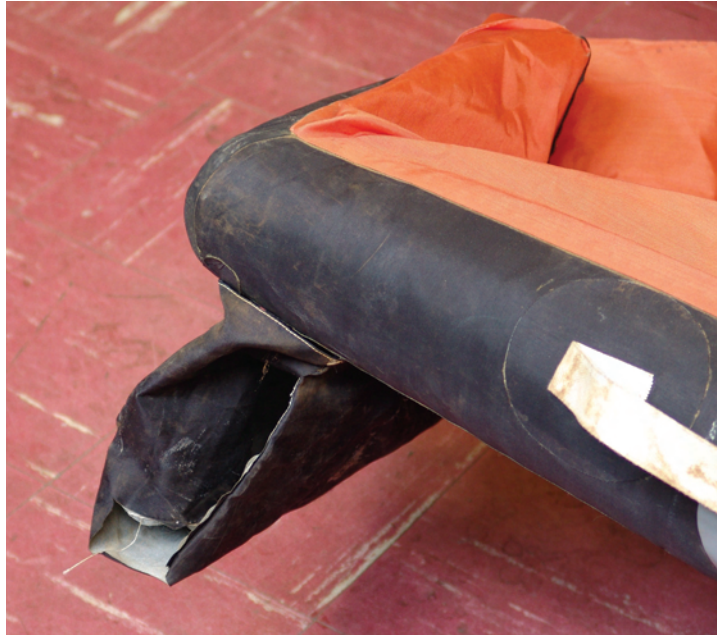
Figure 27: Raft Serial Number 2204171 Forward Stability Pocket Detail
