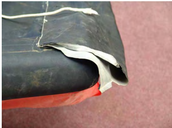
Figure 10: Raft Serial Number 9834882 Forward Stability Pocket Detail
