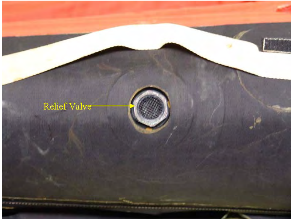
Figure 23: Raft Serial Number 0364812 Over-Inflation Protection Relief Valve
