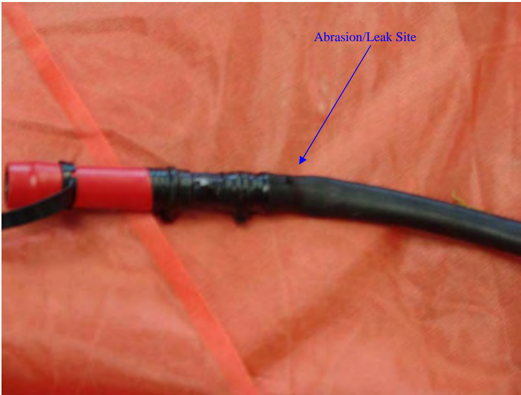
Figure 11: Raft Serial Number 9834882 Manual Inflation Tube Detail
