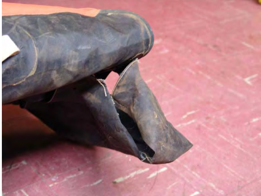
Figure 15: Raft Serial Number 0364837 Forward Stability Pocket Detail
