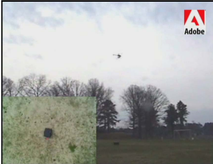
Figure 25. Real Time Flight Video Containing Bottom View of Tracking Desired Hover Location
