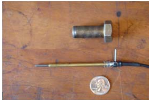
Figure 3. Mounting bolt and laser light probe with fiber optic cable
