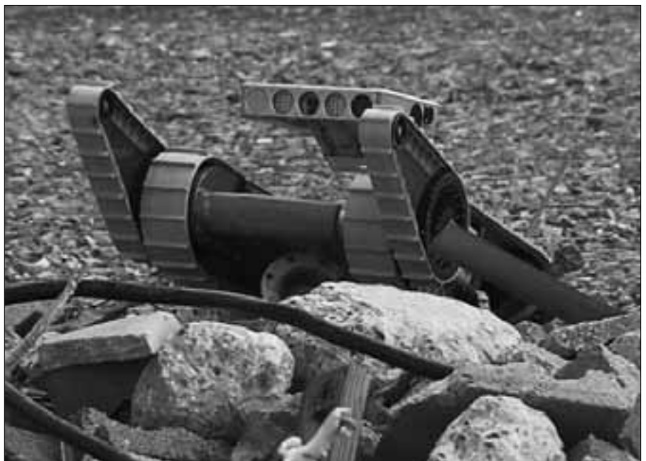
Its optical sensor package in the raised position, a Packbot climbs a debris mound during a Future Combat Systems demonstration last fall. The robotic vehicle is one of the FCS technologies that has been leveraged for the current force. U.S. Army photograph by Steve Harding.
