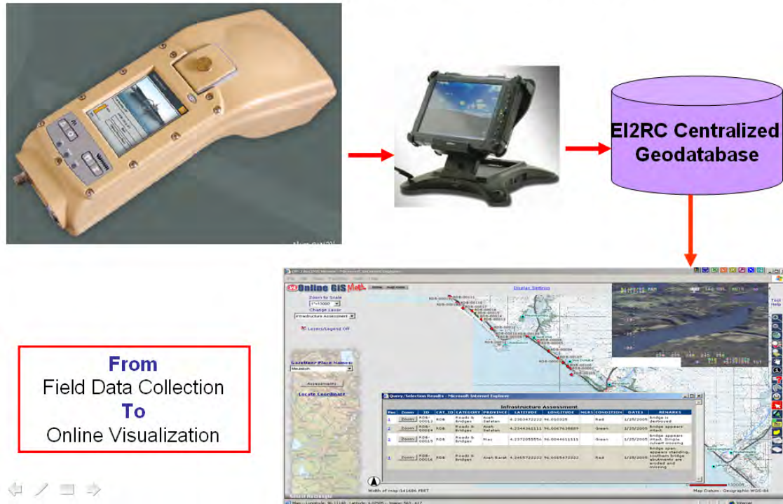
Figure 9. Basic Architecture of the GATER Data Exchange Utilizing the IKE Handheld Device (upper left) and the EI2RC Web Portal (lower right).
