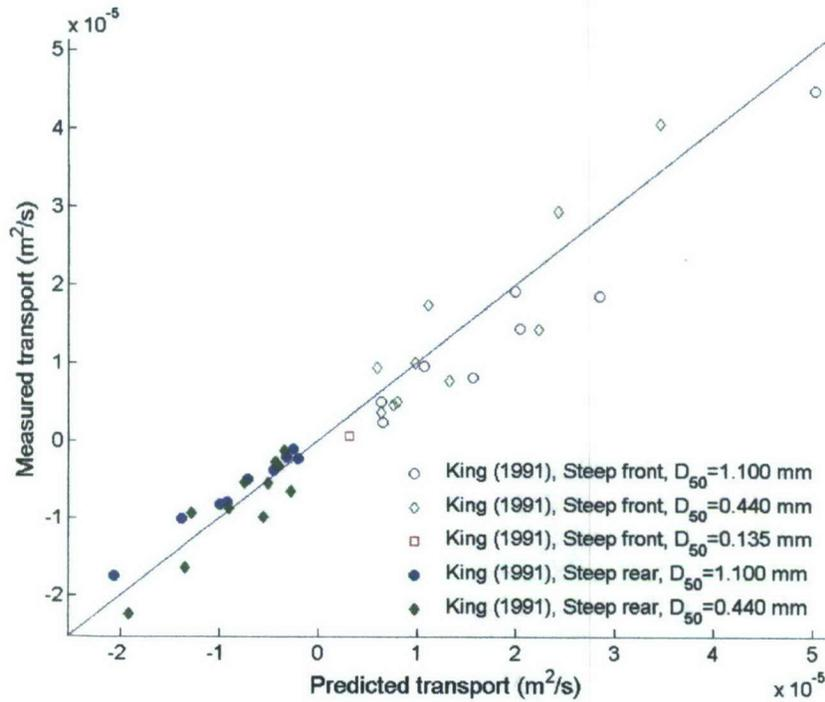
**Figure 5: Comparison between measured and predicted average sediment transport rates under asymmetric and non-skewed waves. Adapted from Gonzalez-Rodriguez and Madsen, 2007. [The measurements correspond to asymmetric waves with steep front and steep rear measured by King (1991). The mean diameters range from 0.44 to 1.1 mm for different experimental cases.]**
