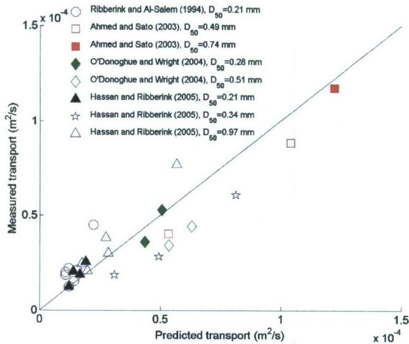
**Figure 6: Comparison between measured and predicted average sediment transport rates under symmetric and skewed waves. Adapted from Gonzalez-Rodriguez and Madsen, 2007. [The measurements correspond to skewed waves measured by different authors. The mean diameters range from 0.21 to 0.97 mm for different experimental cases.]**
