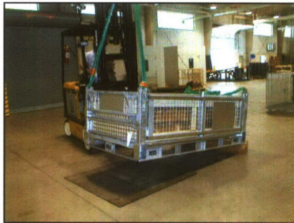
Photo 3. Example of Edgewise-Rotational Drop Test (MSTF Low)
