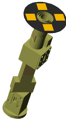
Figure 2-8: Monopulse Antenna System. Photo courtesy of S. Targonski, MIT LL, Group 63
