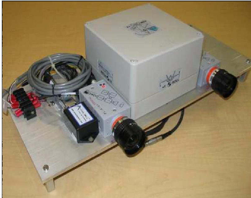
Figure 4.1: Data collection system. The data collection system consisted of a consumer-grade MEMS IMU and monochrome digital cameras. Although not used in this research, a tactical-grade IMU was co-mounted on the platform in order to provide a performance comparison between different grades of inertial sensors.
