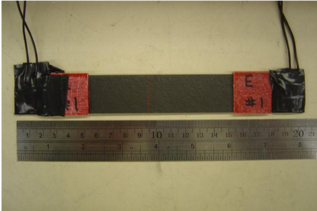
Figure 11. M55J/RS-3 with exterior nickel nanostrands TM tensile specimen.
