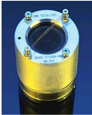
Figure 3. Ion Source with Tungsten Filament Neutralizer 23
