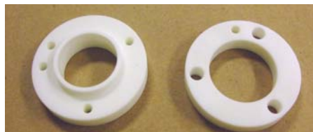
Figure 20. Ceramic Insulators between Keeper and Cathode Base
