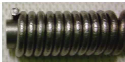
Figure 22. Tantalum Sheathed Heater Wire
