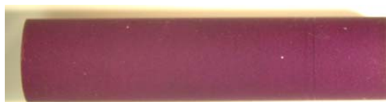
Figure 104. LaB 6 Insert before Testing
