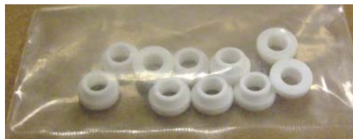
Figure 21. Shoulder Insulators between Mounting Screws and Keeper Electrode
