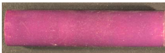
Figure 103. LaB 6 Insert after 52 Hours of Testing
