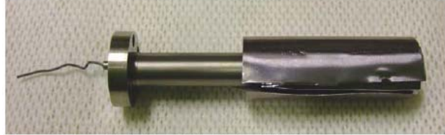
Figure 7. Open Cathode with Radiation Shielding
