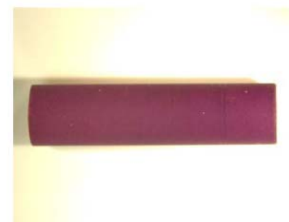
Figure 1. Polycrystalline LaB6 Hollow Cathode Insert
