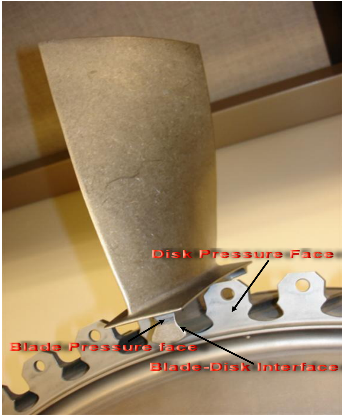
Figure 1.1 Blade/Disk Dovetail Joint in a Turbine Engine
