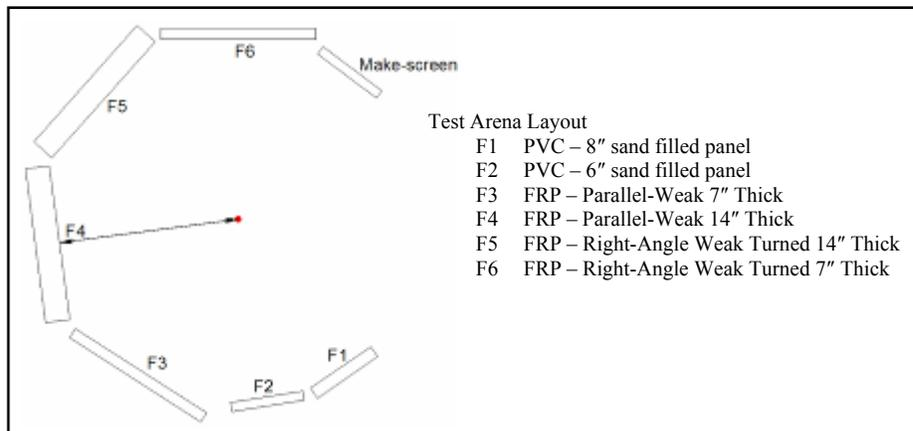
**Figure 9 – Wall Panel Experiment for Fragmentation Setup**
