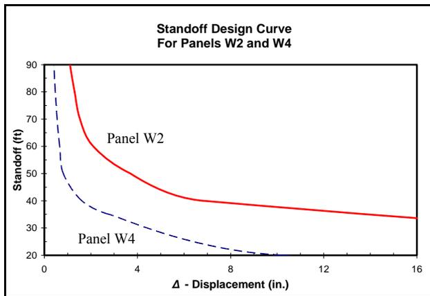
Figure 6 – Wall Panel Test Design Curve
