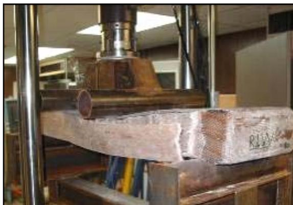
Figure 3 – Four Point Bending of Small-Scale Samples
