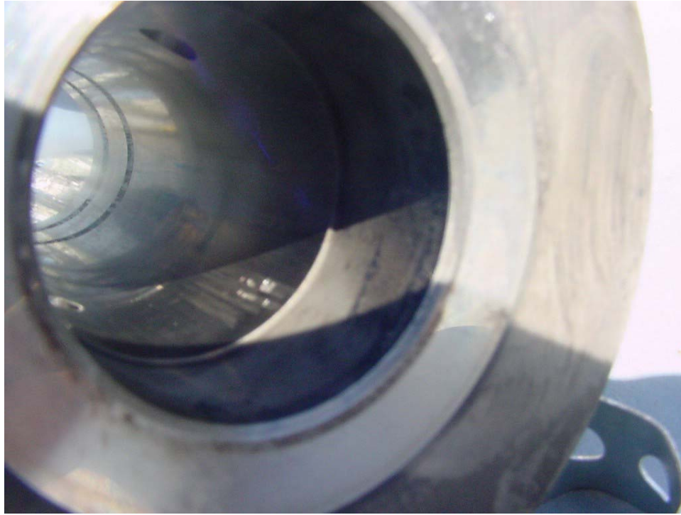
Figure 18. Wear Scars in Injection Pump Barrel
