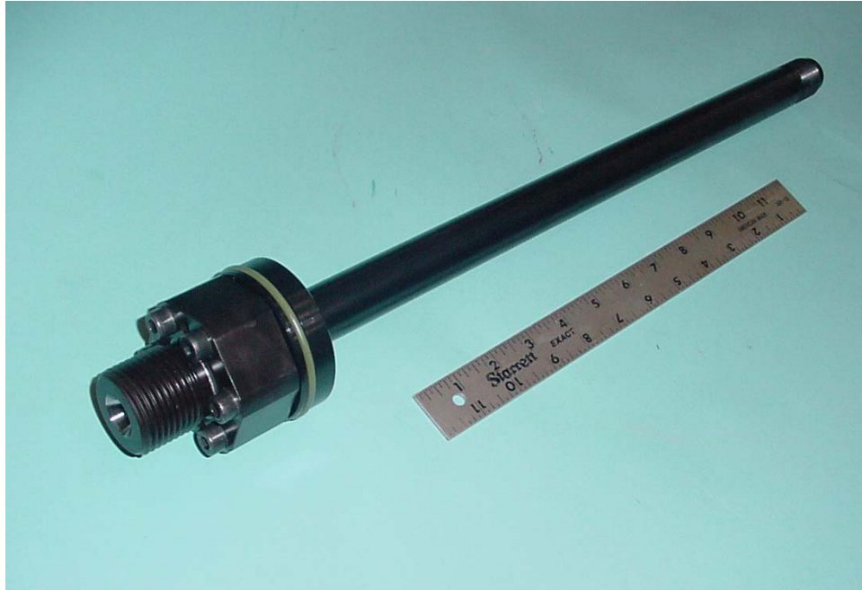
Figure 4. Delivery Valve Holder and Injection Line for 12ZAV40S Engine
