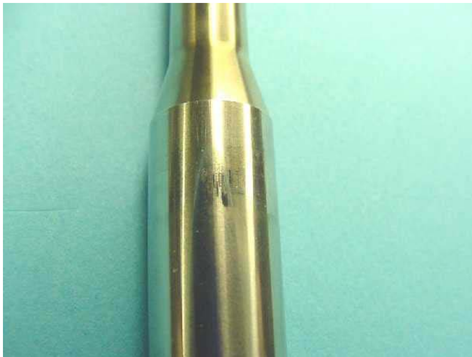
Figure 44. Wear Scar on Fuel Injector Pintle
