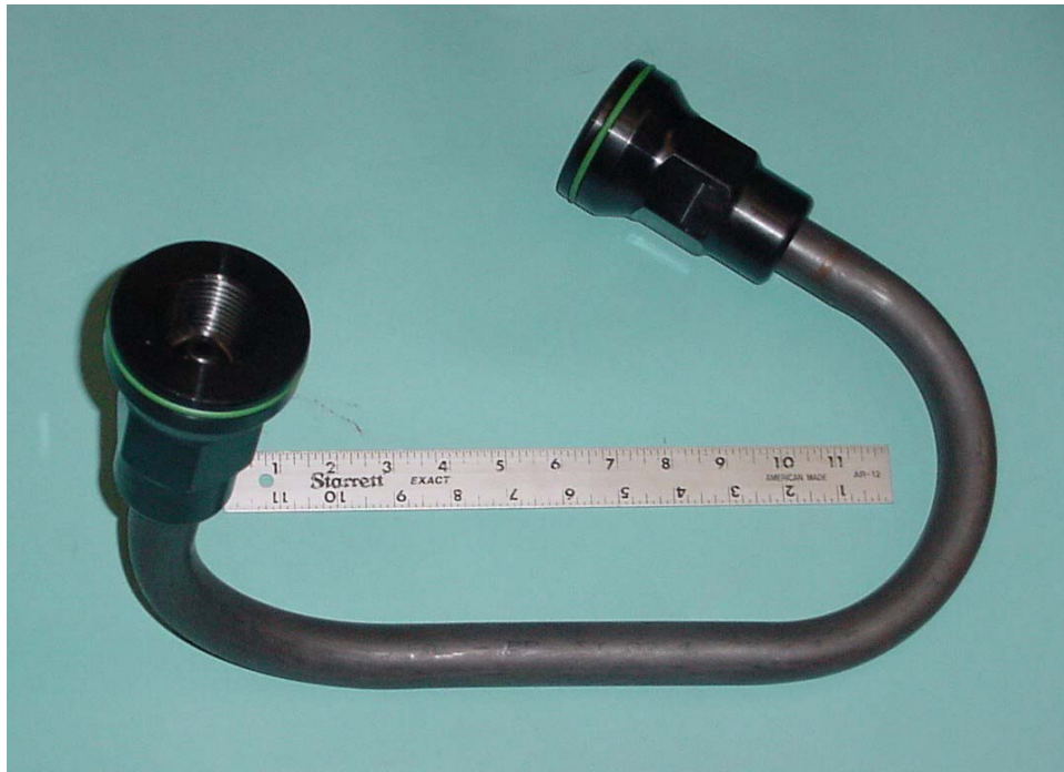
Figure 3. Injection Line for 12ZAV40S Engine
