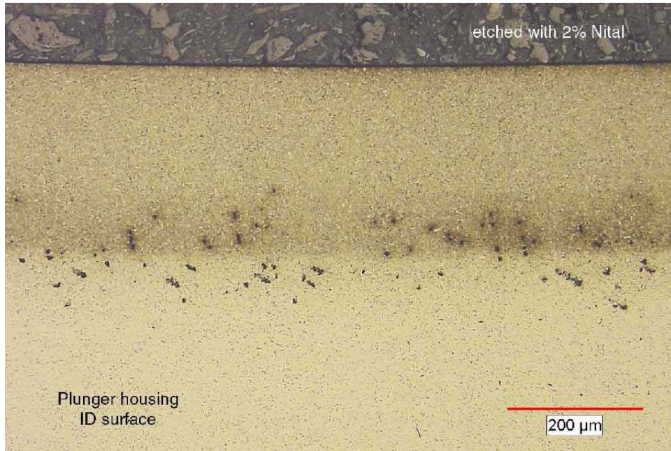
Figure 32. Barrel Etched to Determine Case Hardness Depth
