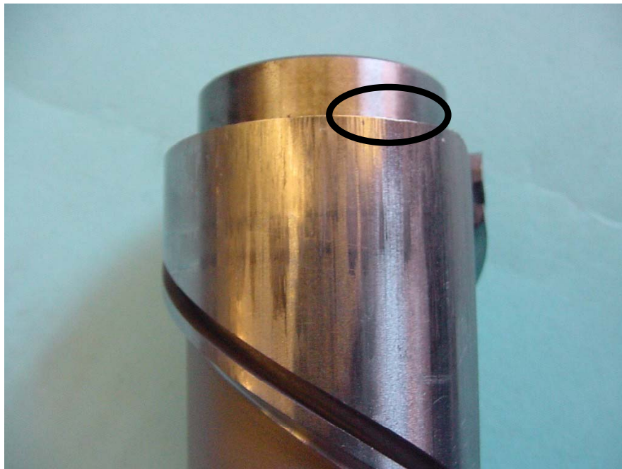
Figure 17. Sulzer Plunger with Wear Scars Formed from Third-Body Wear
