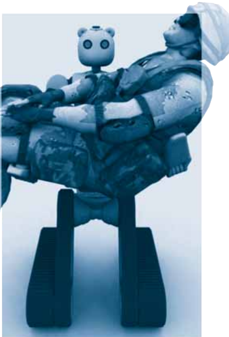
The Battlefield Extraction Assist Robot (BEAR) is designed to rescue wounded troops and reduce the risk to medics.
