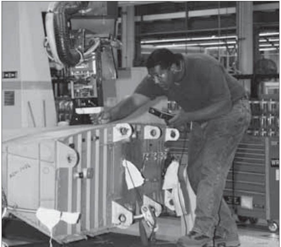
Gene Manns, Air Force sheet metal mechanic, programs the robotic machinery to remove screws from the top panel of an F-15 Eagle wing in the F-15 wing shop at Robins Air Force Base, Ga.
