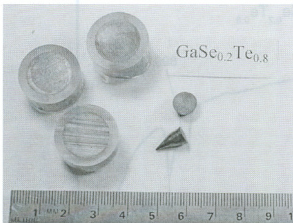
Figure 9. Photograph of a \text{GaSe}_{0.2}\text{Te}_{0.8} crystal after being sectioned with a wire saw.
