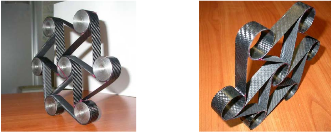
Figure 21 – Composite chiral cell
